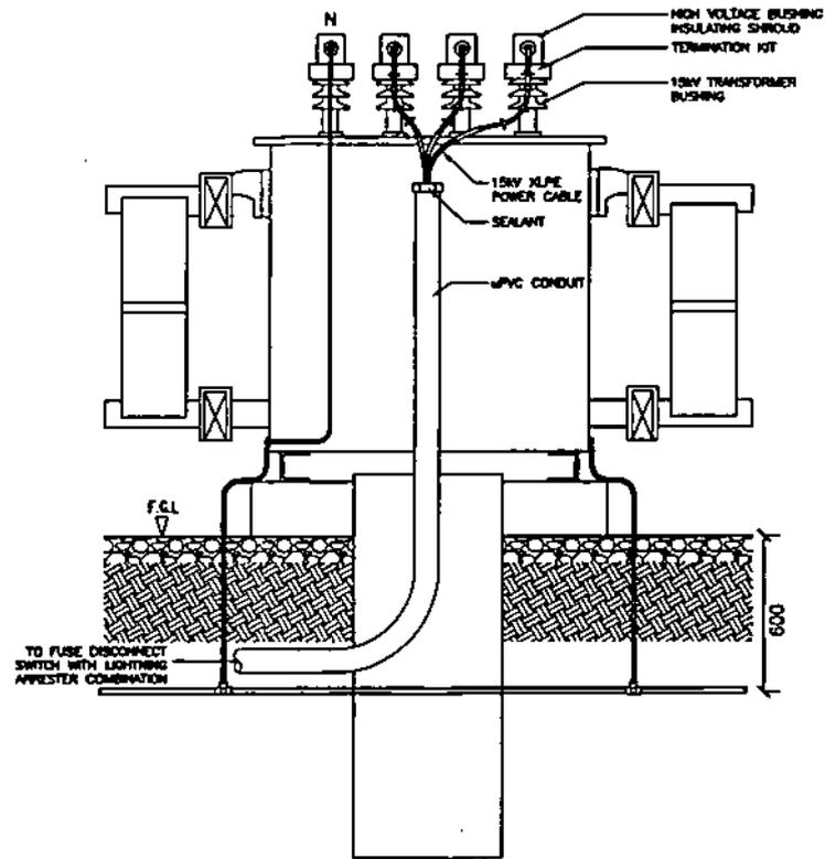
TRANSFORMER HIGH VOLTAGE CABLE TERMINATION
