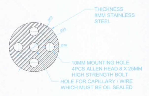
NOTE: 1. FLANGE IS FOR OIL SEALING PURPOSE
